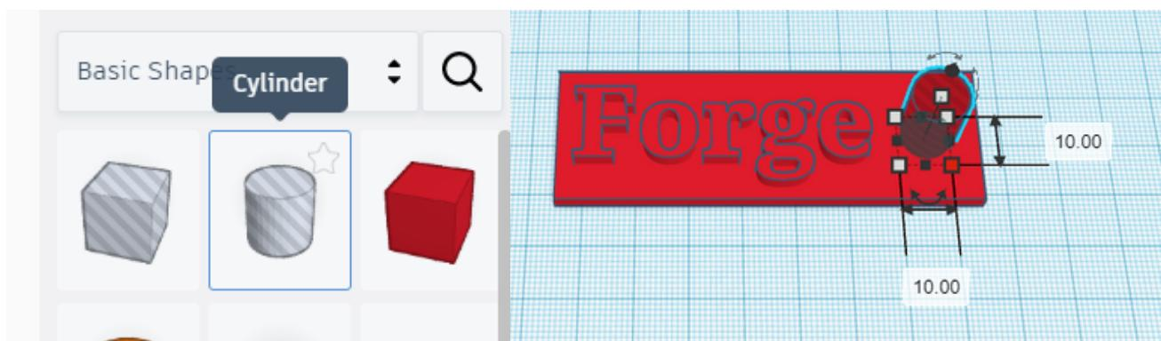
8. Highlight all the components (rectangle, text, and cylindar hole) and press the group tool on the top right.
