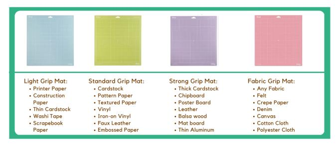
(Going to light of stickiness will have your material lift off the mat and get stuck under the machine, while picking one that too sticky will cause some trouble with removing the material from the material and you might end up ripping it)
