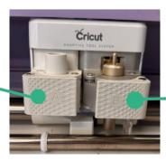
On the right side labeled B is where you can switch out the blades. When you want to switch out a different blade just pull on the tab and carefully take out the blade that in there and insert the new one.
