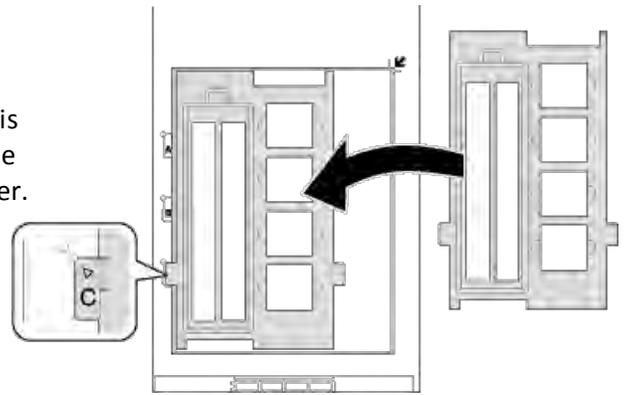
Place up to four slides in the film holder with the shiny base side facing down. Your images should appear backwards on the side that faces up. Your images should be oriented as shown.
