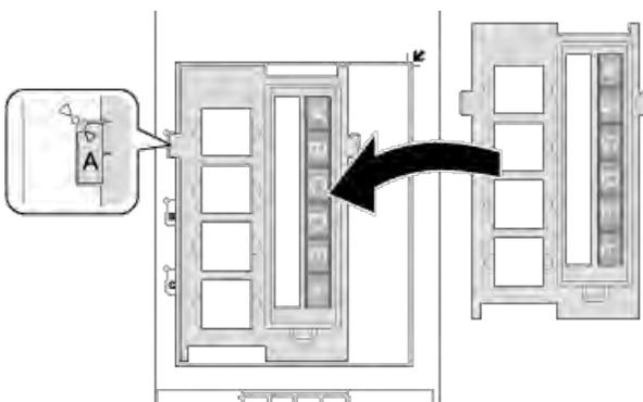
Place the film holder on the document table so that it is aligned with the upper left corner. Make sure the tab labeled "A" on the film holder fits into the area labeled "A" on the scanner.
