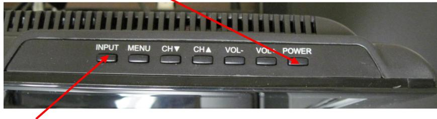
3) Make sure the TV input is set to **HDMI1**. You can check and set this by using the Input button on the top edge of the screen.
